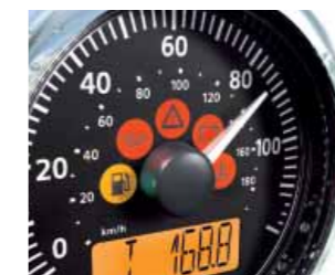
Highly visible LED warning and indicator lights
